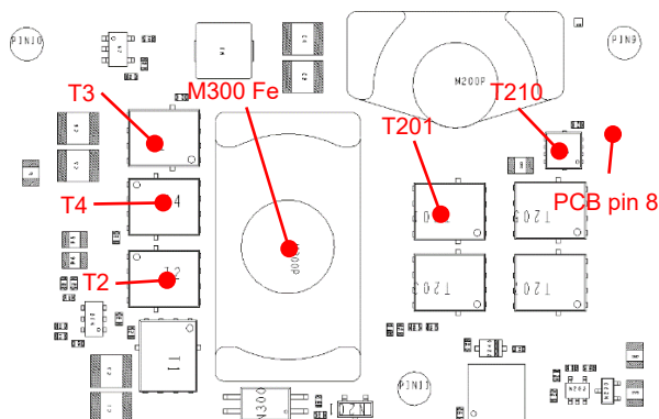
Figure 4. Thermocouple location.
